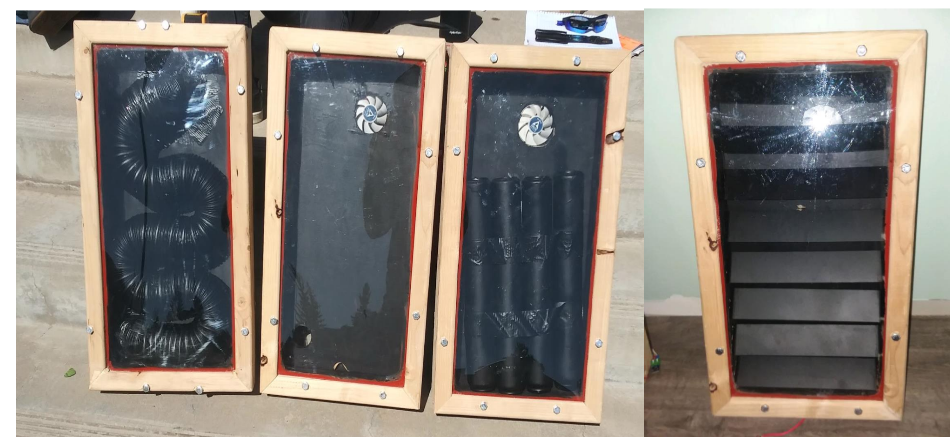
Figure 1: From left to right, ducted solar furnace, control solar furnace, aluminum can solar furnace, and steel shutter model solar furnace prototypes.
